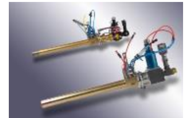
Images of the IPO optics for cladding
